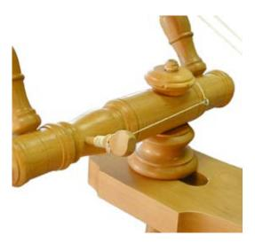
Left - note how Scotch tension is installed.
