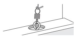
**4.** Rub candle wax onto the end of the screw eye. Thread the screw eye into the pilot hole in the right-hand side.
