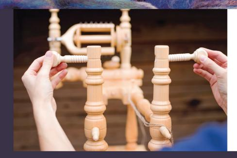
Step 17: Insert the crank thumb screws into the wheel posts.
