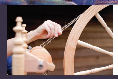
Step 20: Set the drive band along the groove on the drive wheel and around the whorl and bobbin.
