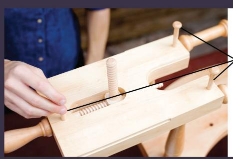
Step 9: Insert locking pegs (3) into holes on top of the table.
