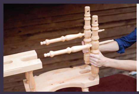
Step 6: Place the two wheel posts into the countersunk holes on the bench.
