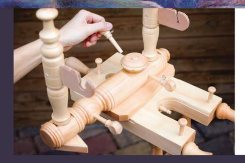
Step 11: Place the Scotch tension and brake pegs into the holes on the Mother-of-all base.
