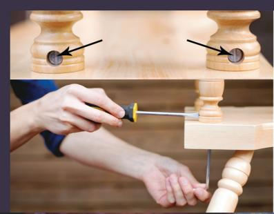
Step 4: Use a screwdriver on nut to help line up hole.
