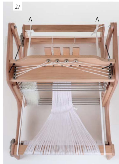
27 Attach 'helping hands' (stretchy cords included in the raddle kit) to the loom. On each side go from the front beam, through the castle, around the back beam, back through the castle and tie at the front beam (see A).
