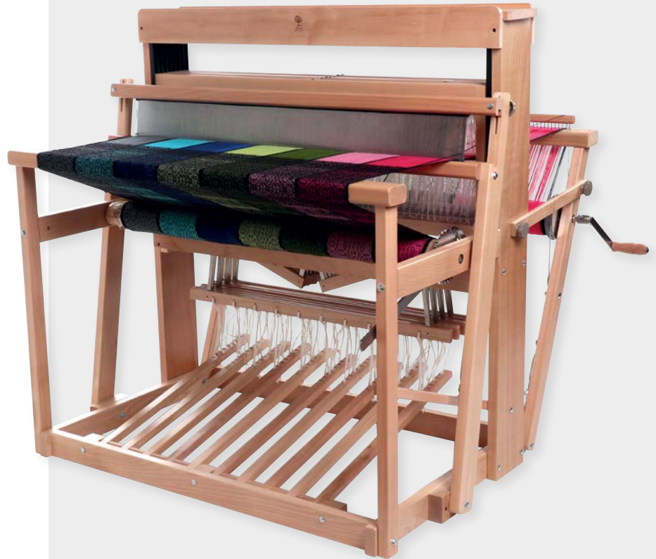
Easy action warp advancement with steel ratchet
