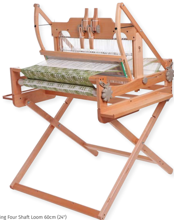
Folding Four Shaft Loom 60cm (24") pictured with optional stand
