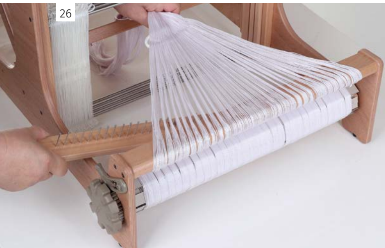
26 Drop the raddle down from the warp.
